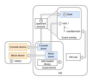
**Figure 2.** VMSH sets up its devices in the guest by side-loading a kernel library. The virtual block device backs the overlay's root. The virtual console handles console input-s/outputs of the spawned process.
