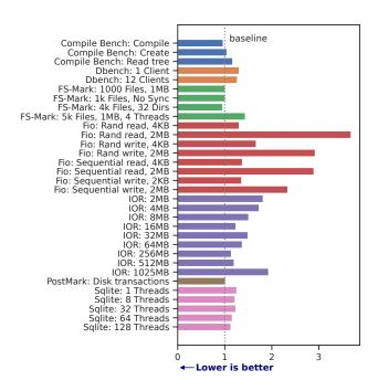
**Figure 5.** Relative performance of vmsh-blk for the Phoronix Test Suite compared to qemu-blk.
