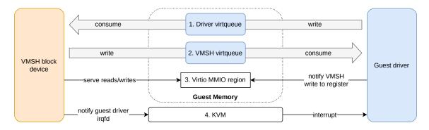
**Figure 4.** VMSH communication infrastructure based on the VirtIO protocol. Guest and host components share data through virtqueues (1, 2). Notification is performed through MMIO regions (3) and KVM (4).
